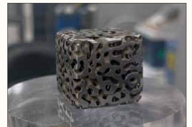
A scaled-up model for visualizing nanoporous metal, a microstructure designed with high stability in a battery.
